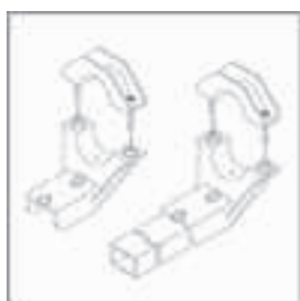
Portafeed con viti premontate Feed holder with pre-mounted screws
